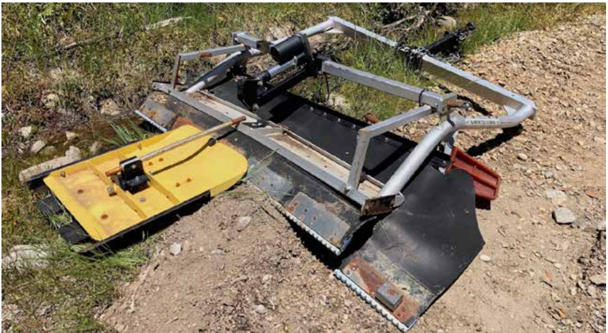
The Ginzugroomer . This was purchased by the Falls Creek Resort to be used in marginal snow conditions when the large Kässbohrer (PistenBully) or Prinoth BR350 could not be used. It could be towed by a snowmobile.
