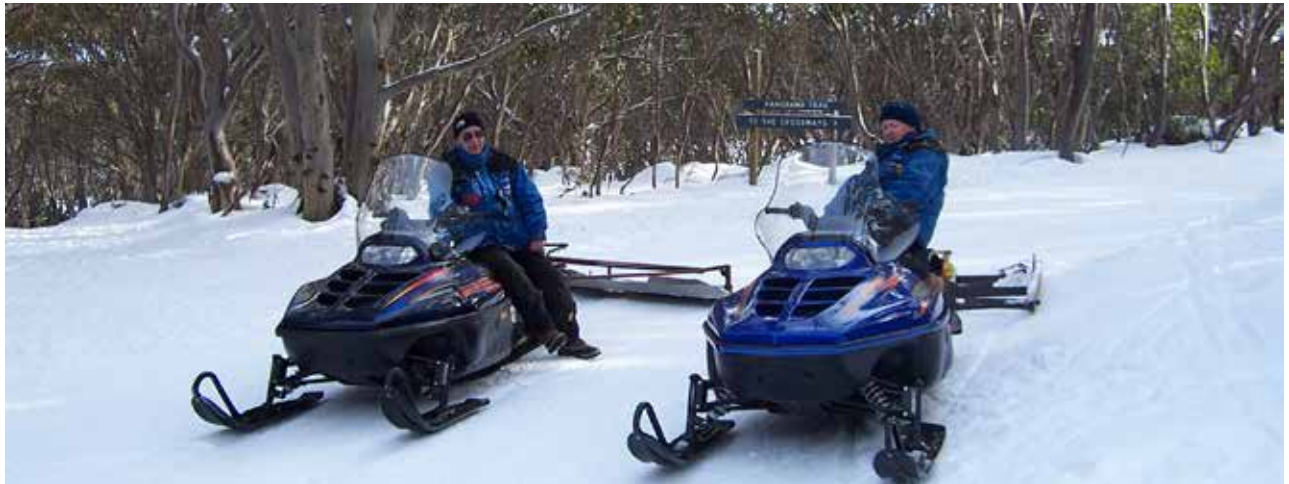
A photo from the late 1990's at Lake Mountain The left snowmobile pulls a 'rut-cutter' with the second snowmobile pulling a 'smoother' that finishes with a bit of a snow-comb effect. Both were home-made devices.
