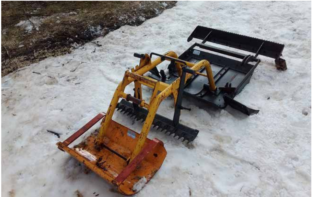
Swiss-made Bachler track-setter with renovator, comb for scrubbing out old tracks and trackplate (at rear on this photo) for laying down the new grooves. It was pulled by a snowmobile. This model of track-setter was also used at Lake Mountain.
