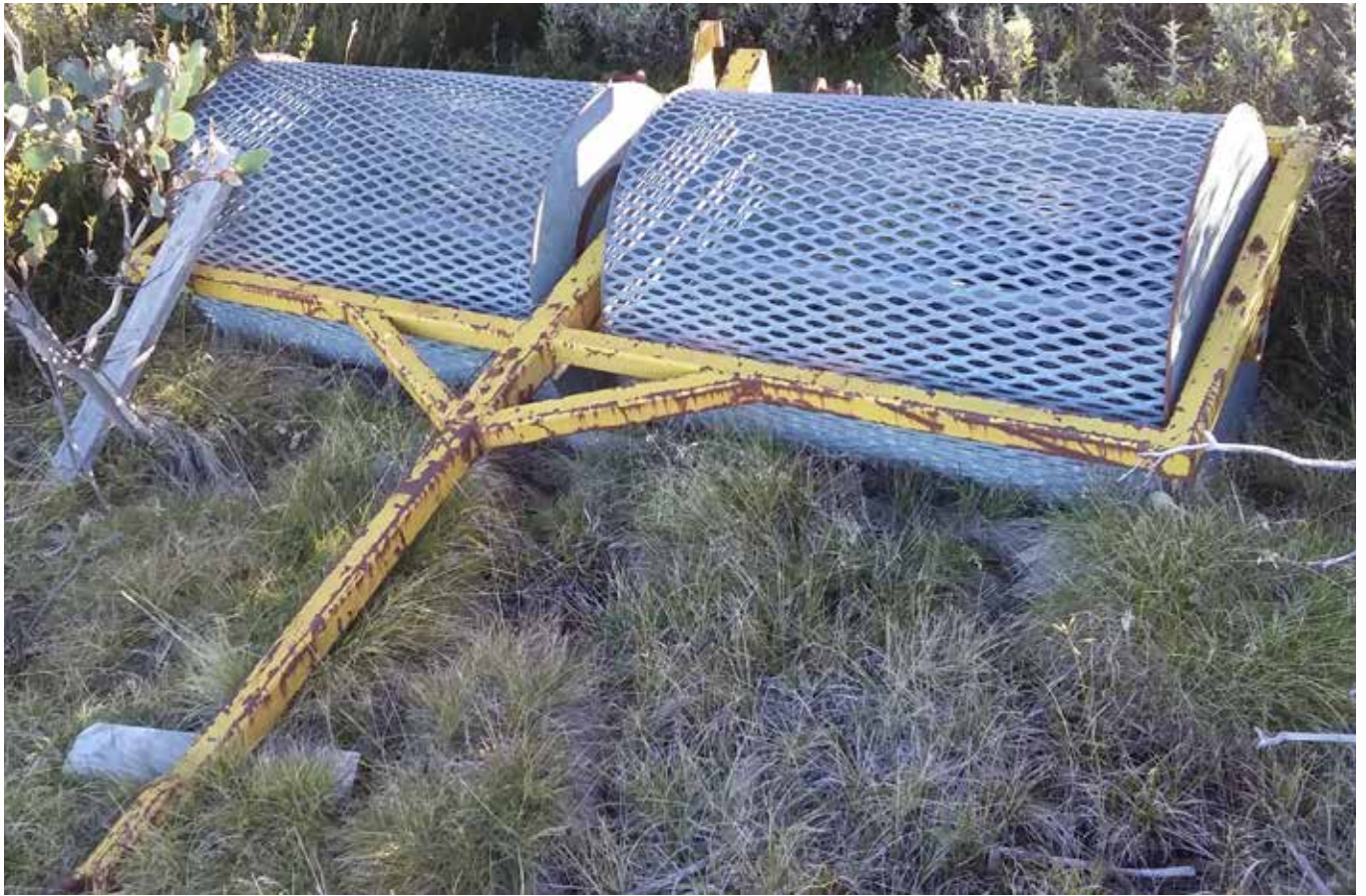
Compactor roller for soft and new snow. It was pulled by a Bombi (see page 4)
