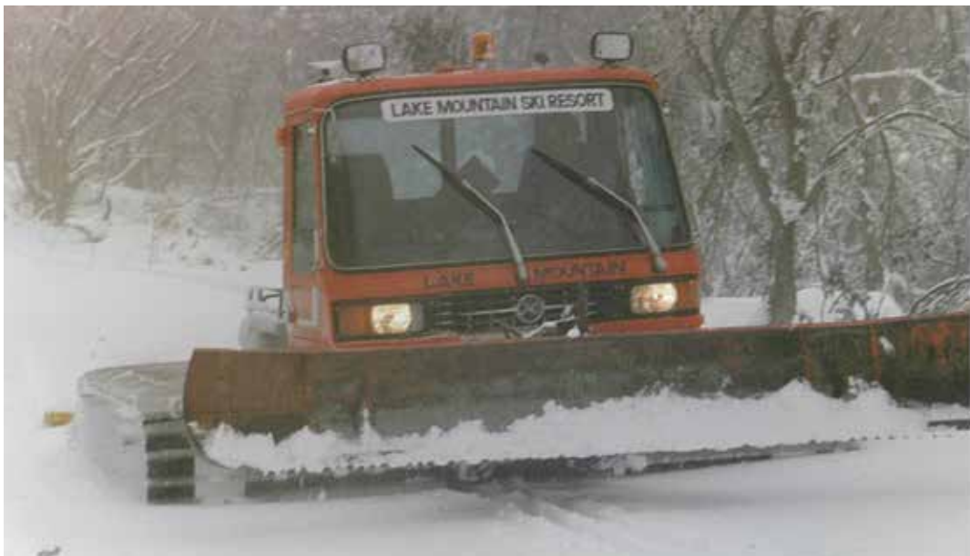
In 1986 a Kässbohrer 170 (PistenBully) was acquired from Mt Hotham. It only had a compactor bar and no tiller. The Bombi or a snowmobile pulling a track setter would follow.
