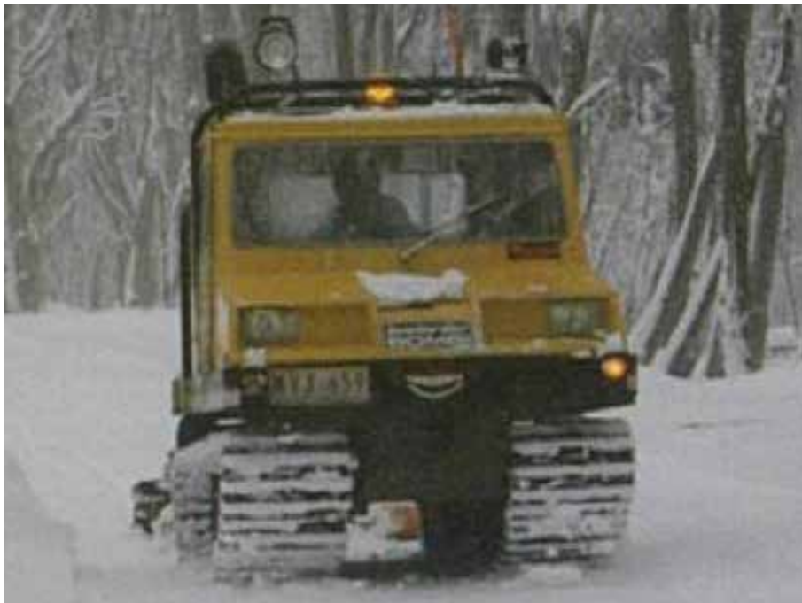
The 1984-acquired Bombardier Bombi compacting the snow. This was followed up with a snowmobile pulling the Swiss Bachler track setter (see page 11). In later years the Bombi (with track setter attached) followed the PistenBully.
